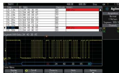
Infrequent LIN parity error captured on the 3000 X-Series in less than a second due to hardware-based serial decode
