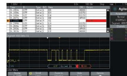
500 CAN serial packets over 9 seconds captured at a high sample rate using the 3000 X-Series segmented memory
